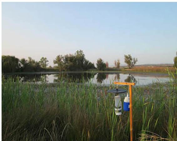
A blue cooler of dry ice emits carbon dioxide, which lures mosquitoes toward a mosquito fan-trap in the Spenceville wildlife area, Yuba County, California.
